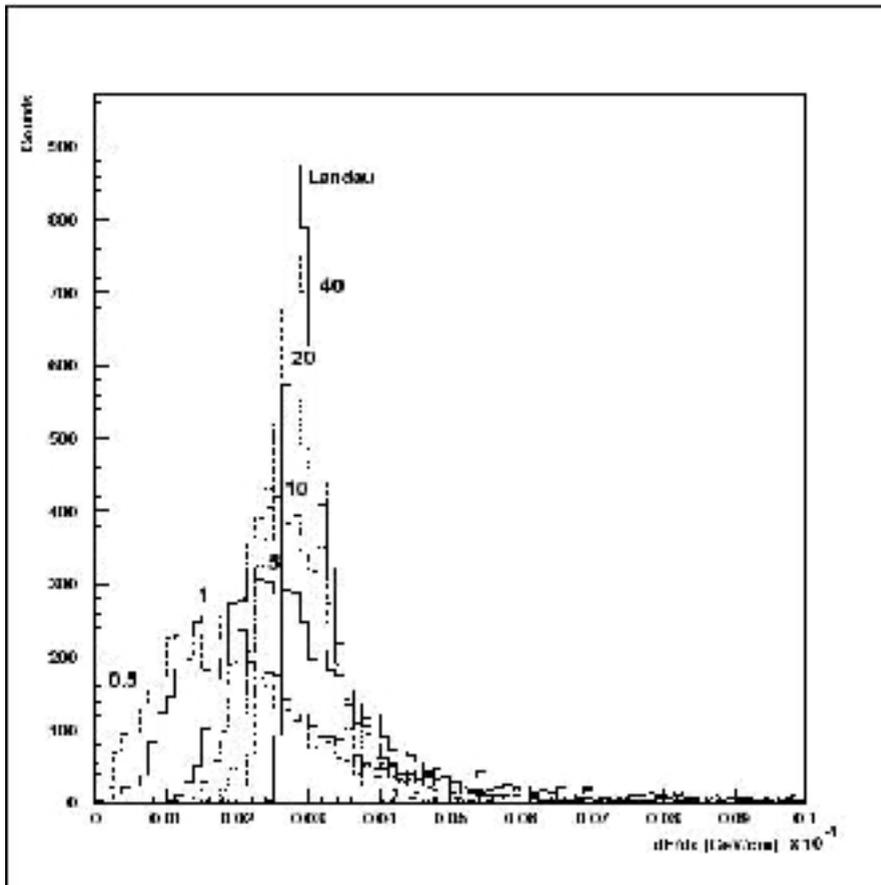
Figure2. Energy loss distribution for a 3 GeV electron in Argon as given by standard GEANT.
