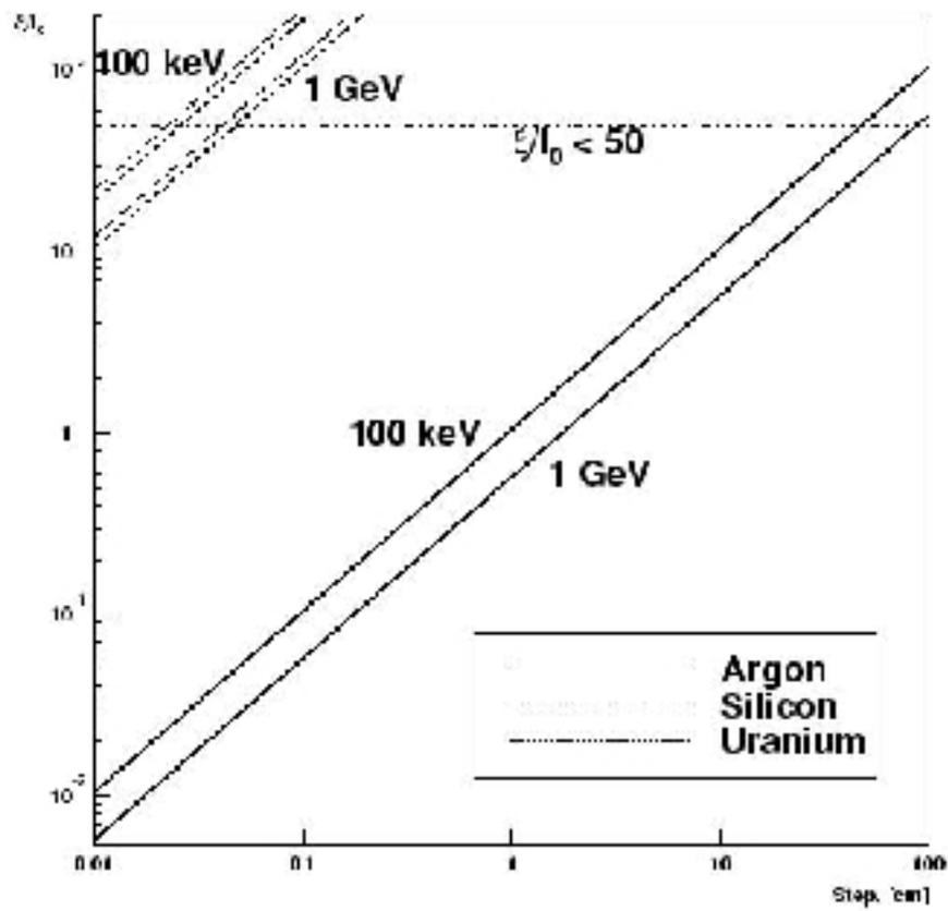
Figure 1. The variable  $\xi/I_0$  can be used to measure the validity range of the Landau theory. It depends on the type and energy of the particle,  $Z$ ,  $A$  and the ionisation potential of the material and the layer thickness.
